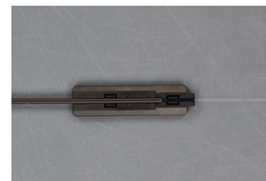
Step 7: Fix the fiber in the cutting jig. The outer jacket must meet the outer jacket limit. The 250µm acrylate coating should meet the end of the cutting jig.
