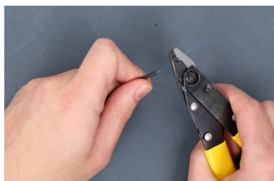
Step 5: Strip off the 250µm acrylate coating back to the added mark—stripping off the mark in the process.
