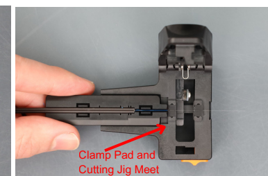
Step 8: Slide the cutting jig in the holder slot of the cleaver until it meets the clamp pad. Cleave fiber.
